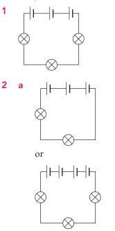
**b** Adding a cell or removing a lamp will increase the current.
